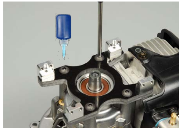
Using the M5 button head bolts secure the mount in place using blue thread lock
