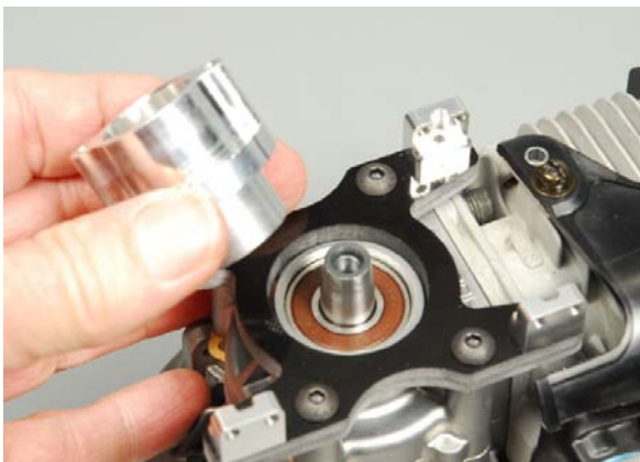
Install the clutch hub on the engine crankshaft as shown
