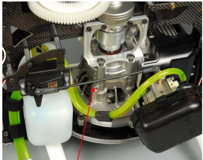
Throttle rod installed
